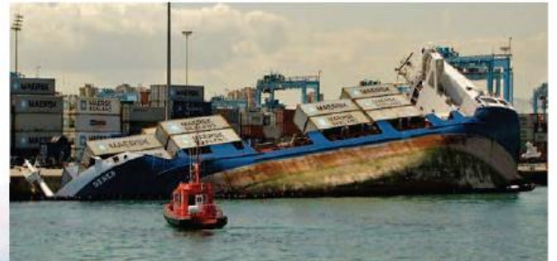
MV Deneb in 2011, rolled over after loading containers where [only] 1 in 10 varied between 1.9 to 6.7 times the declared weight
