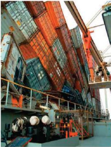
P&O Nedlloyd Genoa suffered a container collapse due to over-weight containers
